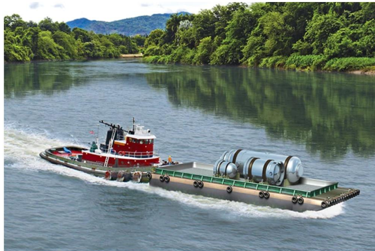
Small modular reactors are designed to be factory-built then transported, as in this illustration. (Supplied: NuScale)
