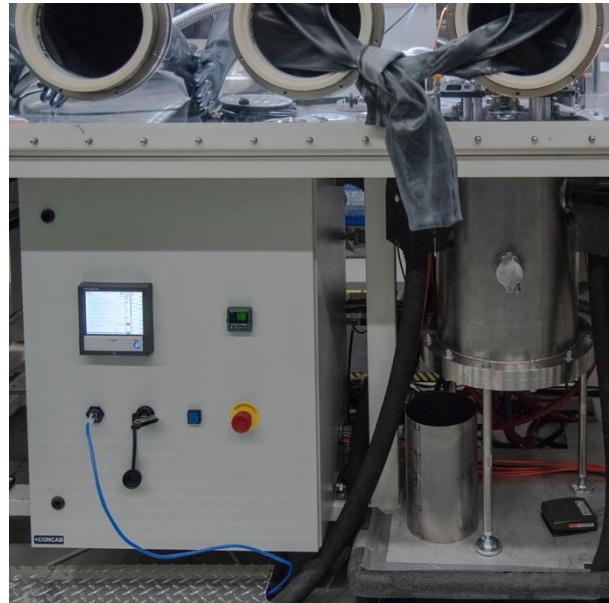
Sintering furnace (EFF) usable hotzone ~4 in x 6 in
