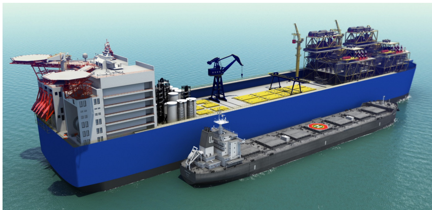
Figure 14. Scenario 2 — FPSO platform for production of synthetic Jet A with bulk carrier arriving alongside for delivery of limestone feedstock. The bulk carrier (smaller vessel on right) drops off the limestone (CaCO 3 ) reagent and picks up lime (CaO) byproduct. Reagents and byproducts are stored in the hull of the FPSO close to the calcination equipment in the stern.
