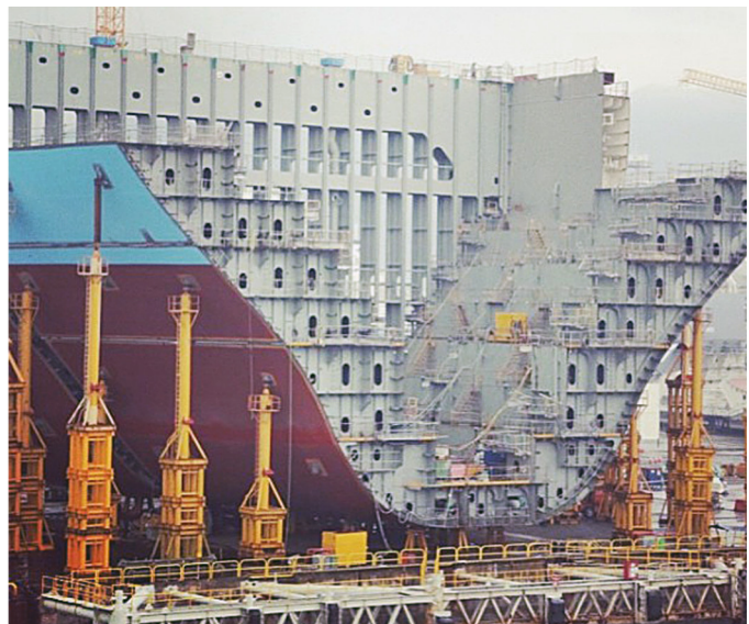
Figure 2. Modular construction. Modular construction is the industry standard for shipyard-based fabrication and assembly. Shown here is a Maersk Triple-E class vessel under construction, at the DSME shipyard in Okpo, South Korea. Used with permission according to Creative Commons terms. By Maersk Line - Flickr photo page, CC BY-SA 2.0, https://commons.wikimedia.org/w/index.php?curid=27646189 .
